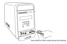
3 If the media does not insert easily, remove it from the slot and verify that it is not upside-down or backwards. Carefully reinsert the Memory Stick media, but do not force it into the slot.
